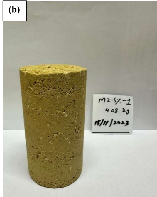
Figure 27. UCS sample preparation (a) AM elements layer (b) UCS cylindrical sample
