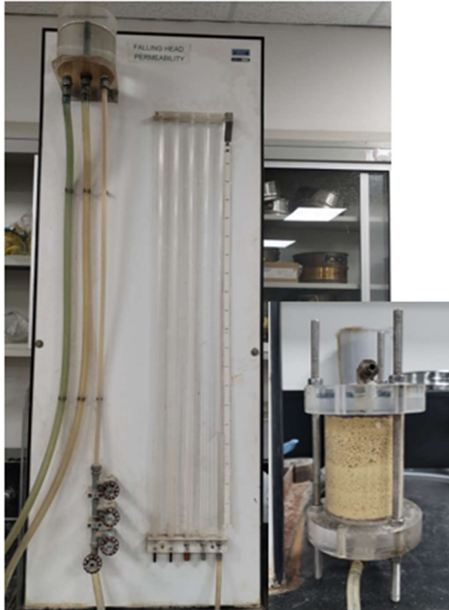
Figure 33. Falling head test apparatus and prepared soil sample
