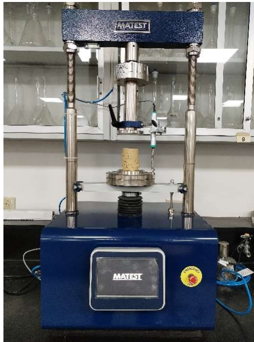
Figure 30. MATEST machine used for unconfined compressive strength tests
