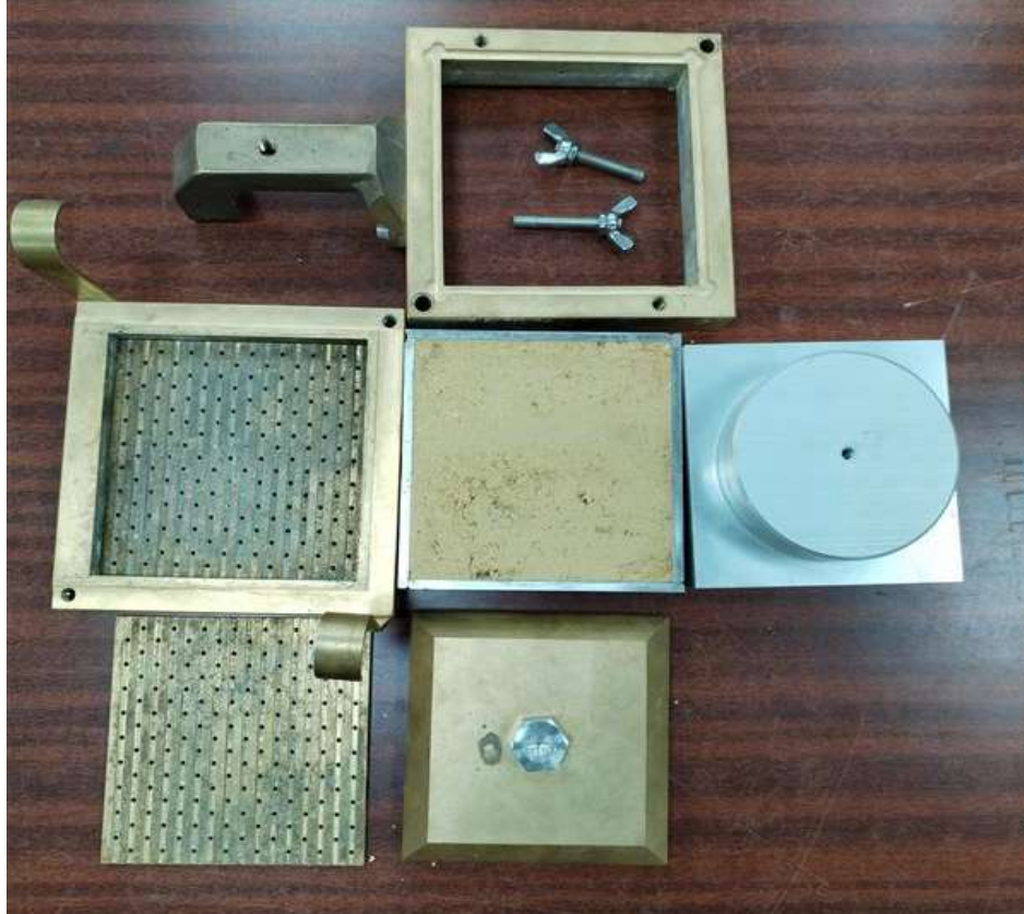
Figure 32. Sampler for direct shear test sample preparation
