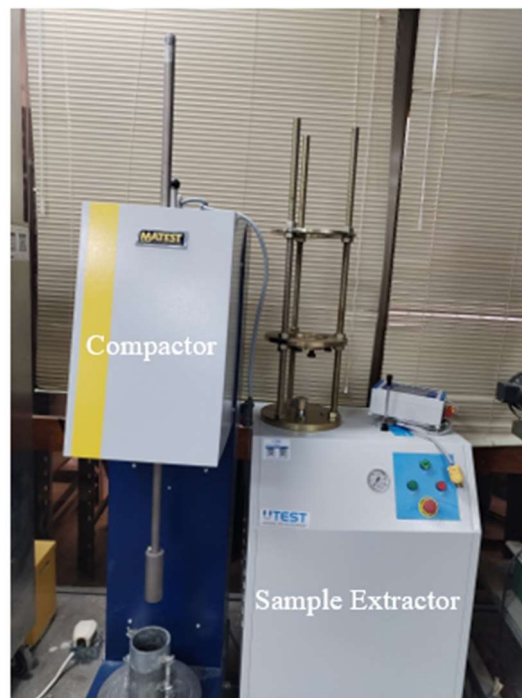
Figure 36. Compacting machine for modified proctor test and sample extractor
