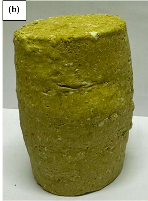
Figure 47. Failure pattern from triaxial test (a) Marl soil (b) AM + soil
