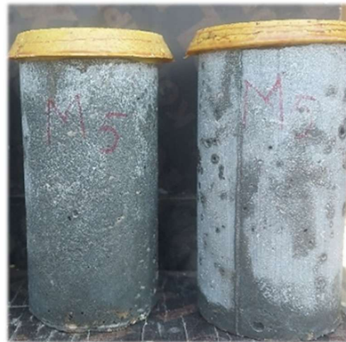
Figure 22. 75 × 150 mm cylindrical specimens (Sulfur capped before compressive testing).
