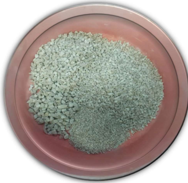
Figure 9. Coarse aggregate of 1/2 in, 3/8 in, 3/16 in, and 3/32, clockwise respectively.
