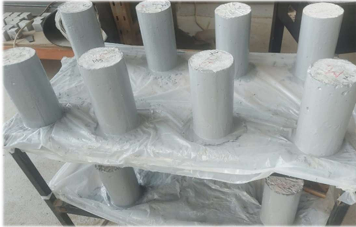
Figure 31. Applying epoxy on the specimen for chloride migration test.
