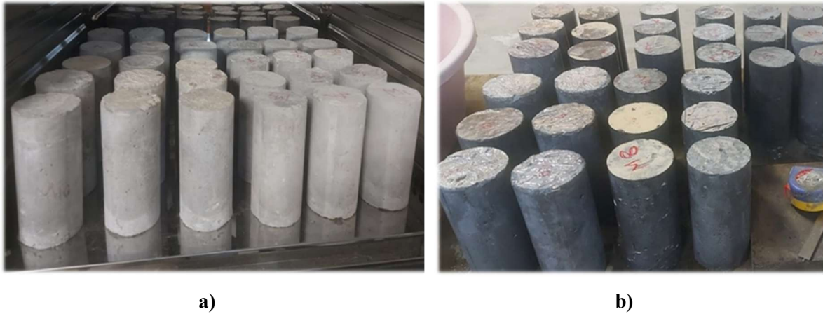
Figure 29. a) Oven drying of concrete specimens was set at 110 °C for 24 hours. b) Concrete specimens in SSD condition.
