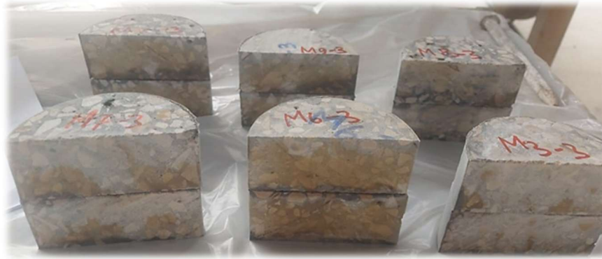
Figure 34. Slicing and applying the silver nitrate ( \text{AgNO}_3 ) for measuring the penetration depth after 24 hours of running the chloride migration test.
