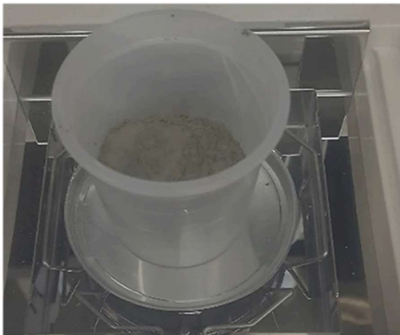
Figure 15. Measuring the weight of the dry sample before mixing.
