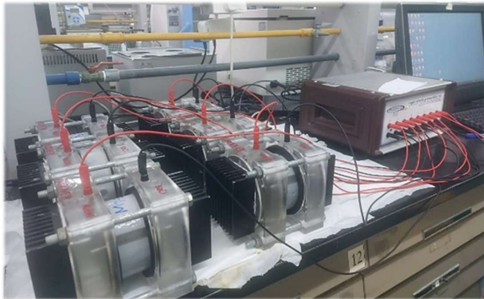
Figure 33. Setting up the disks for running the chloride migration test
