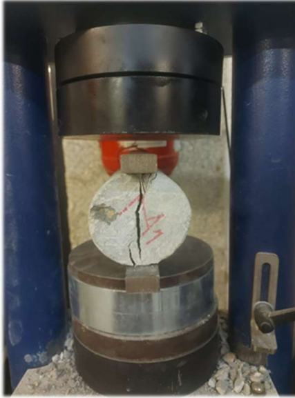
Figure 27. A cylinder specimen under split tensile test.
