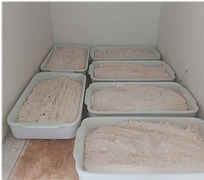
Figure 6. Calcination of clay at 700 °C.
