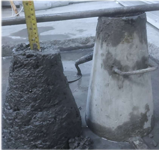
Figure 23. Slump test of the mixture without SP.
