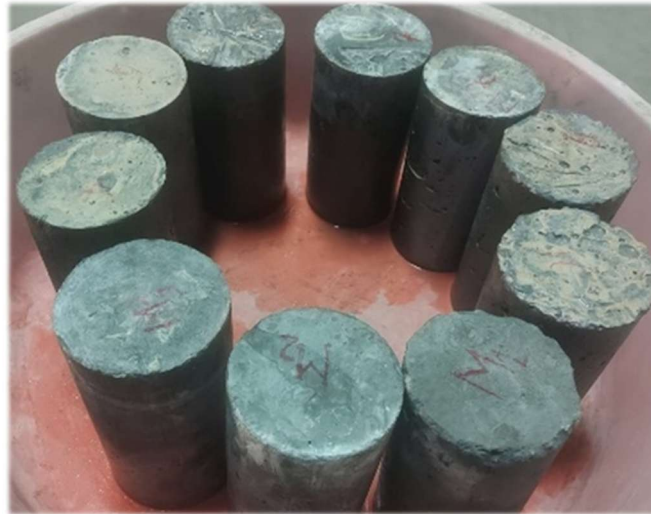
Figure 30. (100 × 200 ) mm, cylindrical specimens for chloride migration test.
