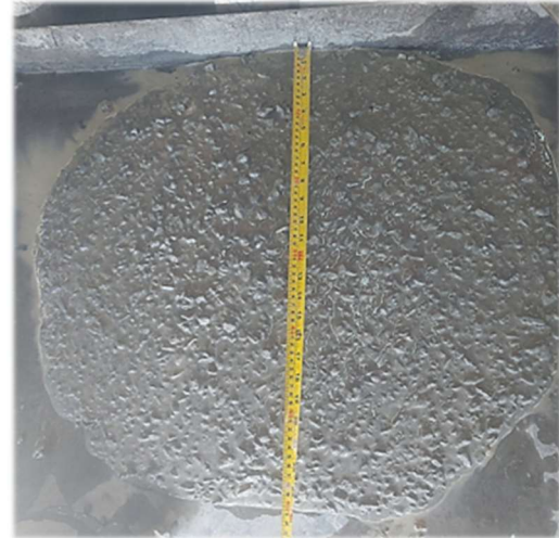
Figure 24. Slump flow test of the developed mixture with SP.
