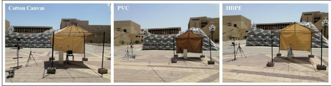
Figure 21: The three different covering materials setting of artificial shades.
