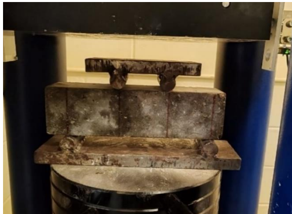
Figure 7: Strength test (Flexural)
