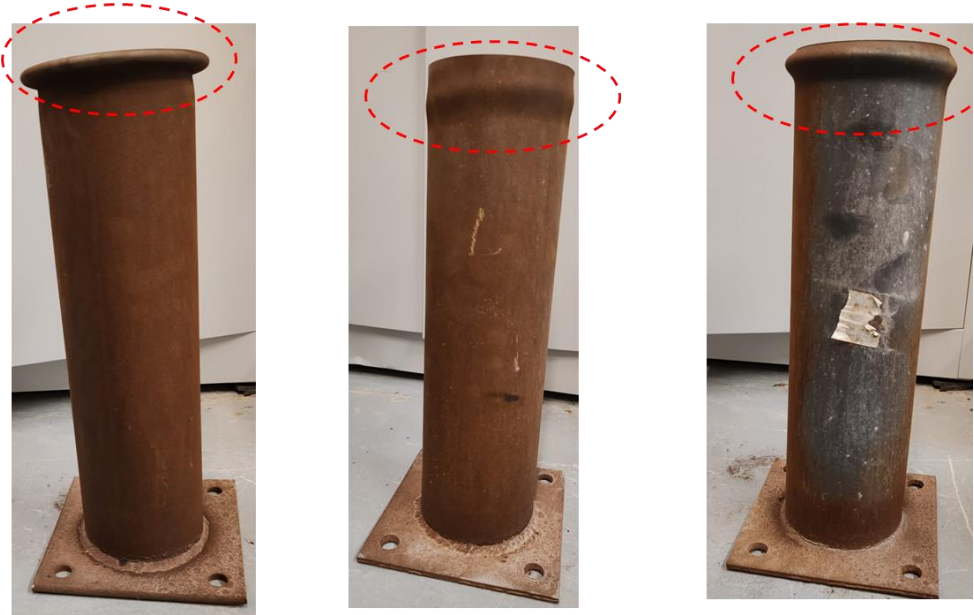
Figure 49: Failure modes of the empty steel tubes
