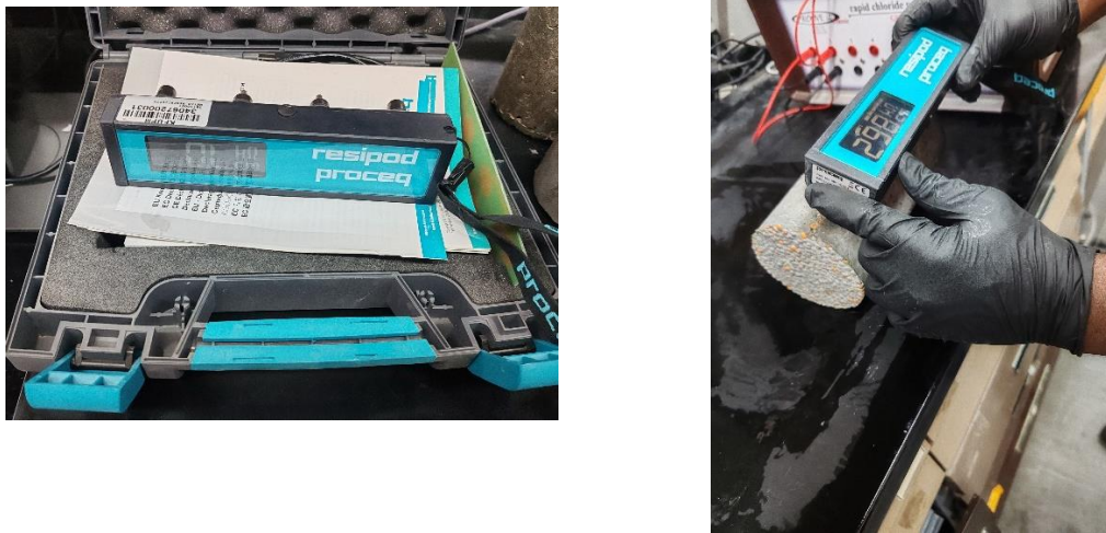
Figure 21: Proceq device and electrical resistivity test on concrete sample
