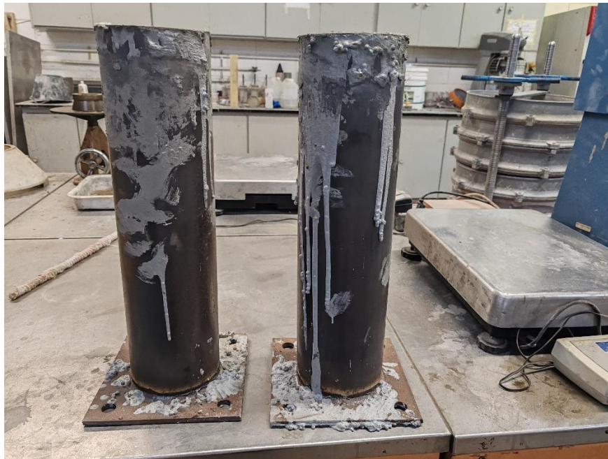
Figure 44: Concrete steel tubes samples after casting
