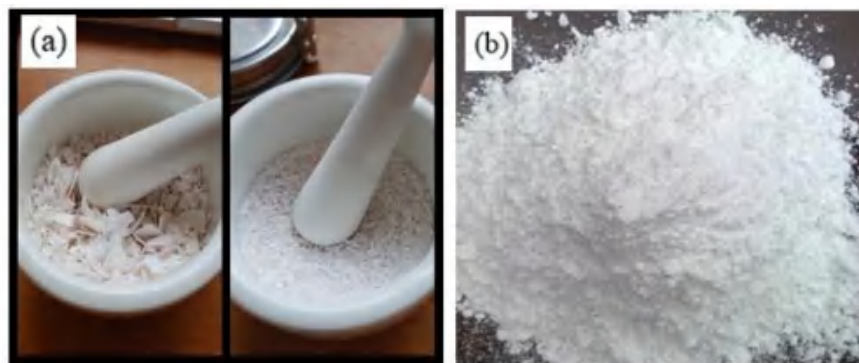
Figure 21. (a) Mortar & pestle grinding eggshells, (b) Eggshell powder.
