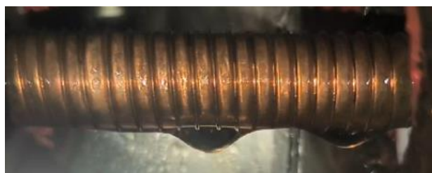
Figure 16 Visual observation of the condensate film at 4 different pitches.
