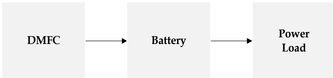
Figure 4: Structure of DMFC/ battery hybrid system in series configuration
