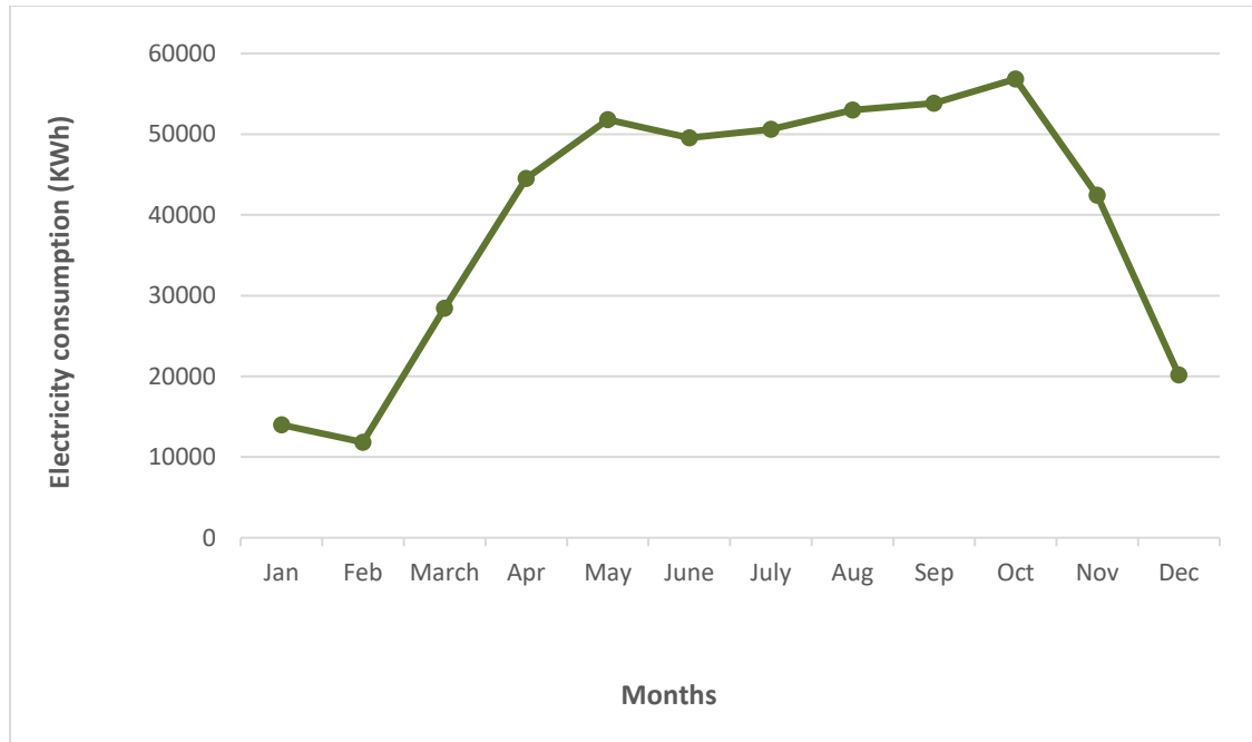
Figure 32 Cooling electricity consumption for case A&B
