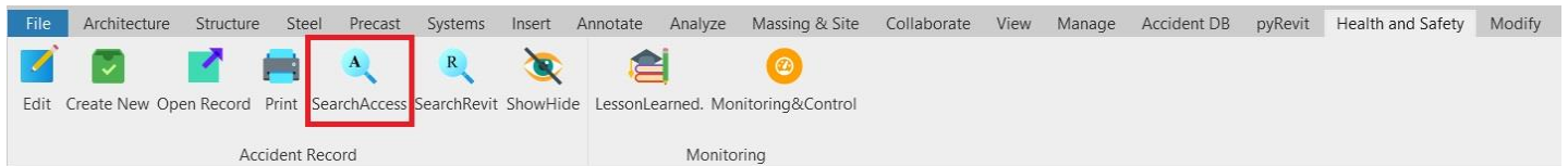
Figure 23: Search access pushbutton
