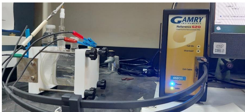
Figure 3.8 Potentiostat setup used for corrosion testing
