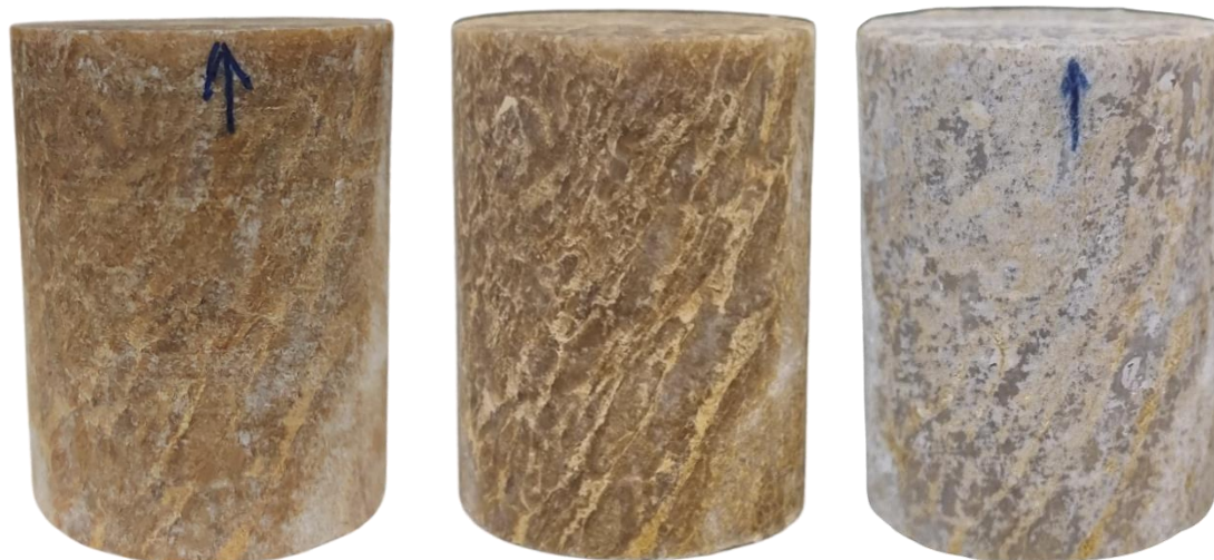
Figure 36. Rock sample before and after supercritical CO 2 -brine interactions; (a) before treatment, (b) after CO 2 -brine treatment, (c) after CO 2 -brine+SrCl 2 treatment.
