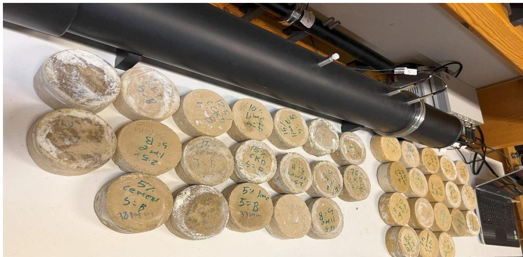
Figure 23. unstabilized and stabilized Hejaz soil specimens alongside their corresponding measurement of BSWA Impedance
