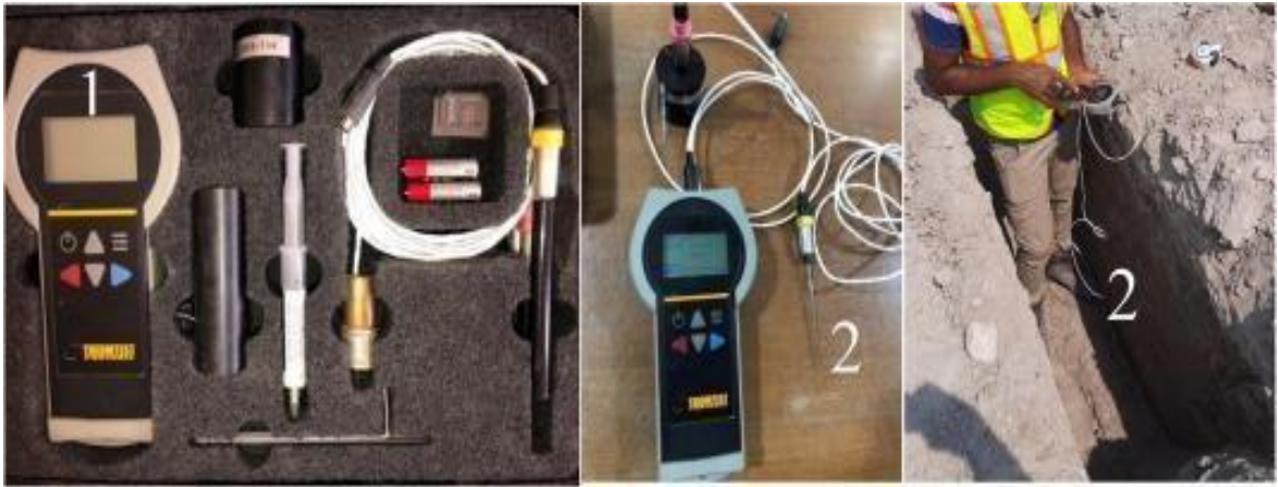
Figure 13. TLS-100 measurements of thermal properties of unstabilized Iraqi soil (field test) [71].
