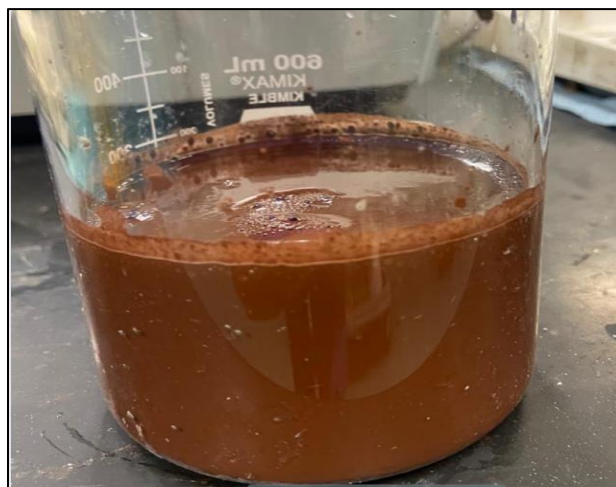
Fig.77: Hyperbranched polymers utilizing \text{Mn}_3\text{O}_4 in high salt formulations show no phase separation after aging at 300 °F
