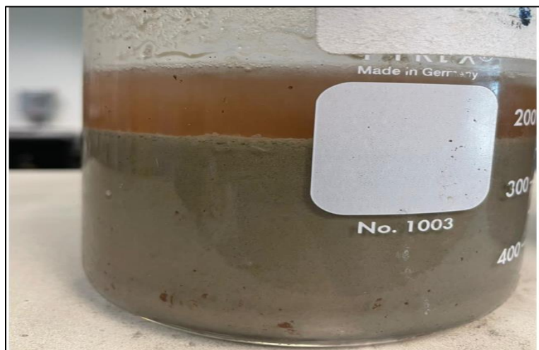
Fig.76: Hyperbranched polymers in high salt formulations show phase separation after aging at 300 °F
