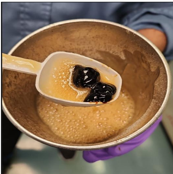
Fig.28: Complete drying of hybrid polymer leads to composite that has little solubility in
