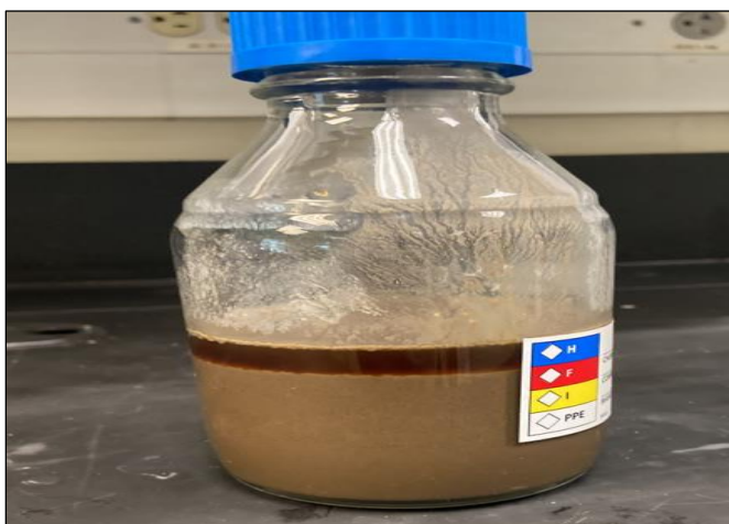
Fig.80: Hyperbranched polymers utilizing Barite in high \text{CaBr}_2 formulations show no phase separation after aging at 300 °F
