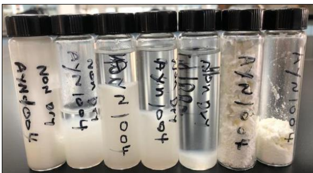
Fig.23: There was a sever phase separation of the nano silica materials AYN1004
