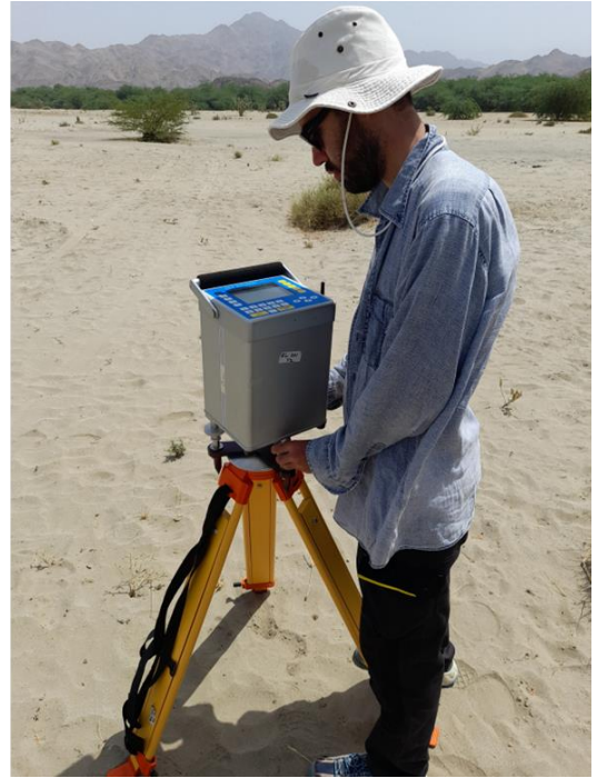
Figure 11: Field photographs of the CG-5 gravimeter during the Wadi Al Lith surveys.
