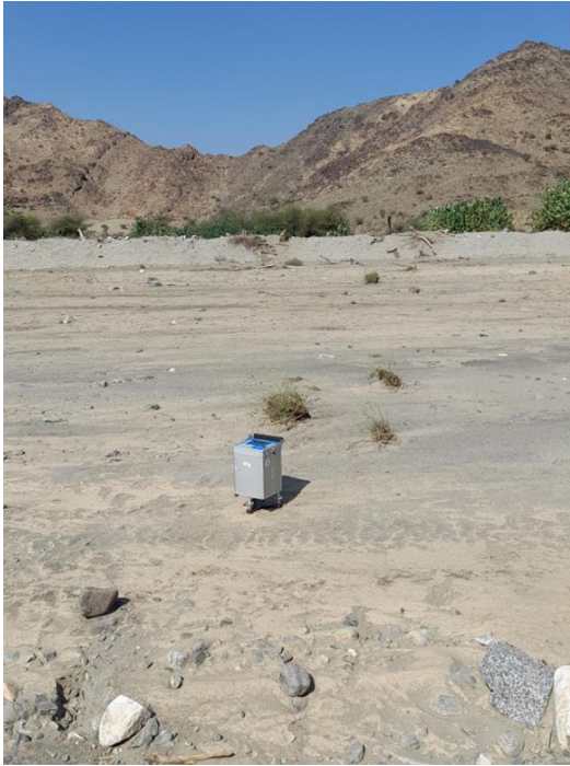
Figure 11: Field photographs of the CG-5 gravimeter during the Wadi Al Lith surveys.
