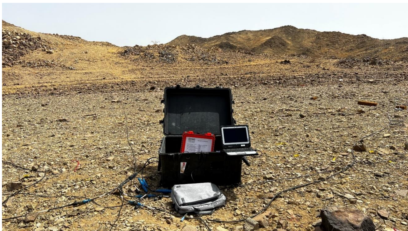
Figure 15: A deployed MT station during the Wadi Al Lith surveys.
