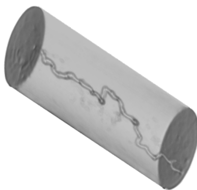
Figure 68 3D image of the induced channel sample W1.
