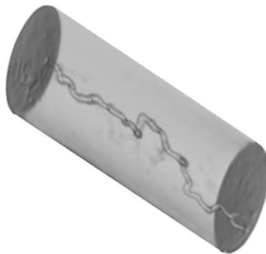
Figure 43 A CT scan of the sample with induced channel.
