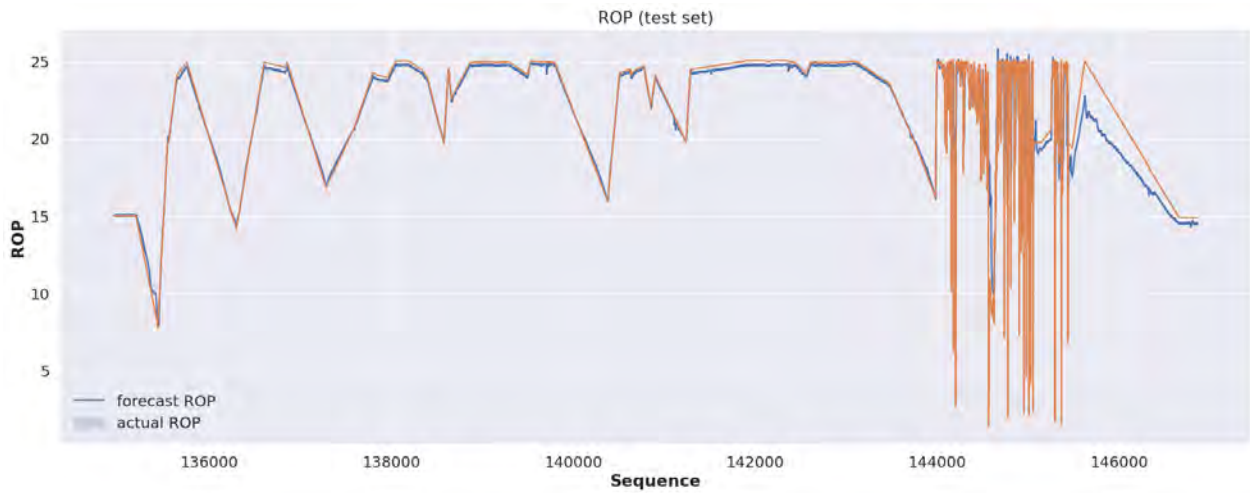
Figure 5.6: Prediction vs Test DROP Chart for Time Based Data Above Depth 3800m
