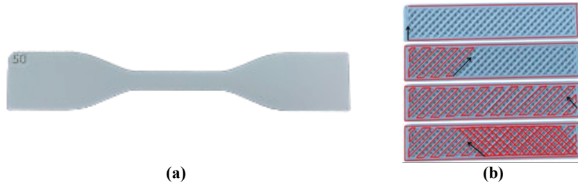
Figure 3.2: (a) Printed PLA FDM sample with 50% infill density and (b) toolpath for internal rasters.
