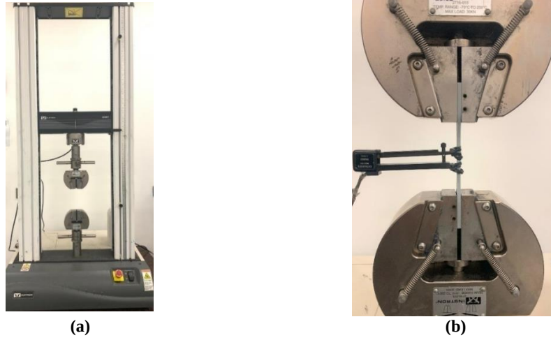
Figure 3.4: (a) Instron® 3367 Universal Testing System for tensile tests and (b) Instron® Catalogue 2620-601 12 mm extensometer.
