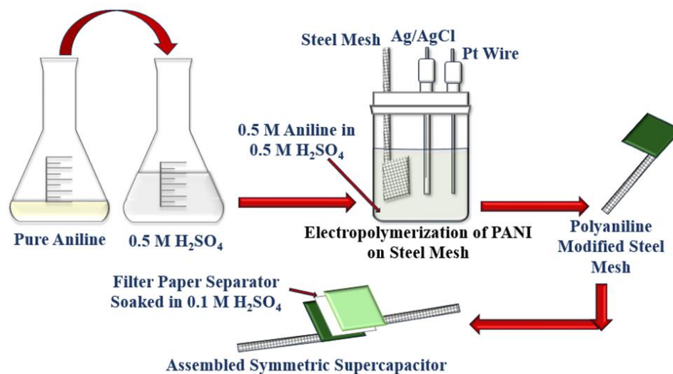
Figure 3.1 An illustrative representation of the process of electrochemically depositing PANI on woven steel meshes of different porosity and the subsequent assembly of a symmetric supercapacitor using the PANI-coated woven steel mesh electrodes
