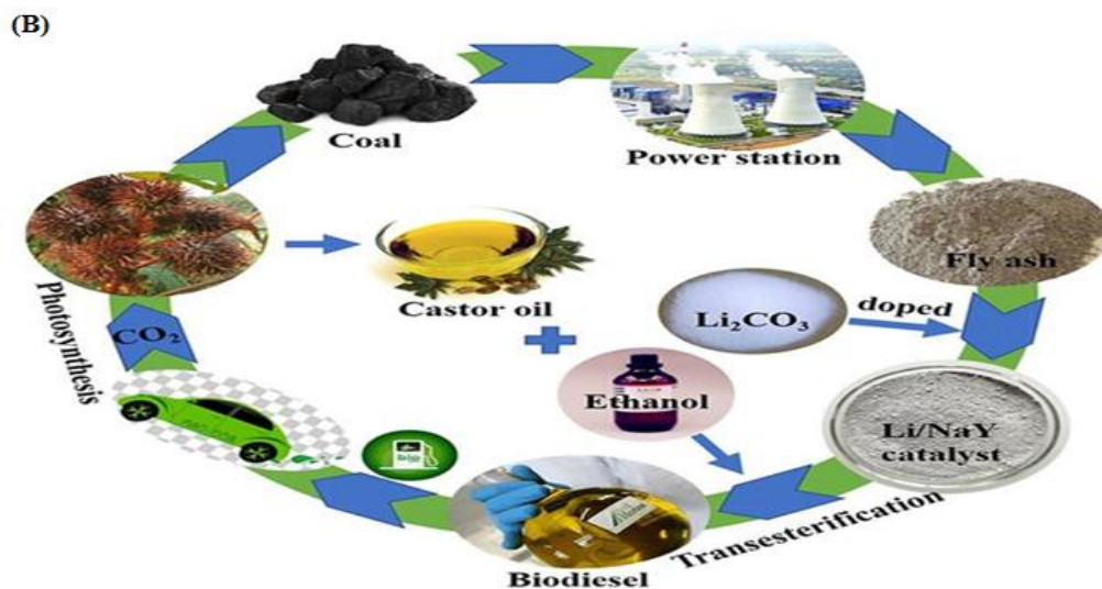
Figure 2.6 (A) Schematic diagram for (a-d) synthesis of Li/NaY zeolite catalyst and (e) structure of Li/NaY zeolite catalyst. (B) Castor oil transesterification using a Li/NaY zeolite catalyst. (Reprinted from ref. 118.)
