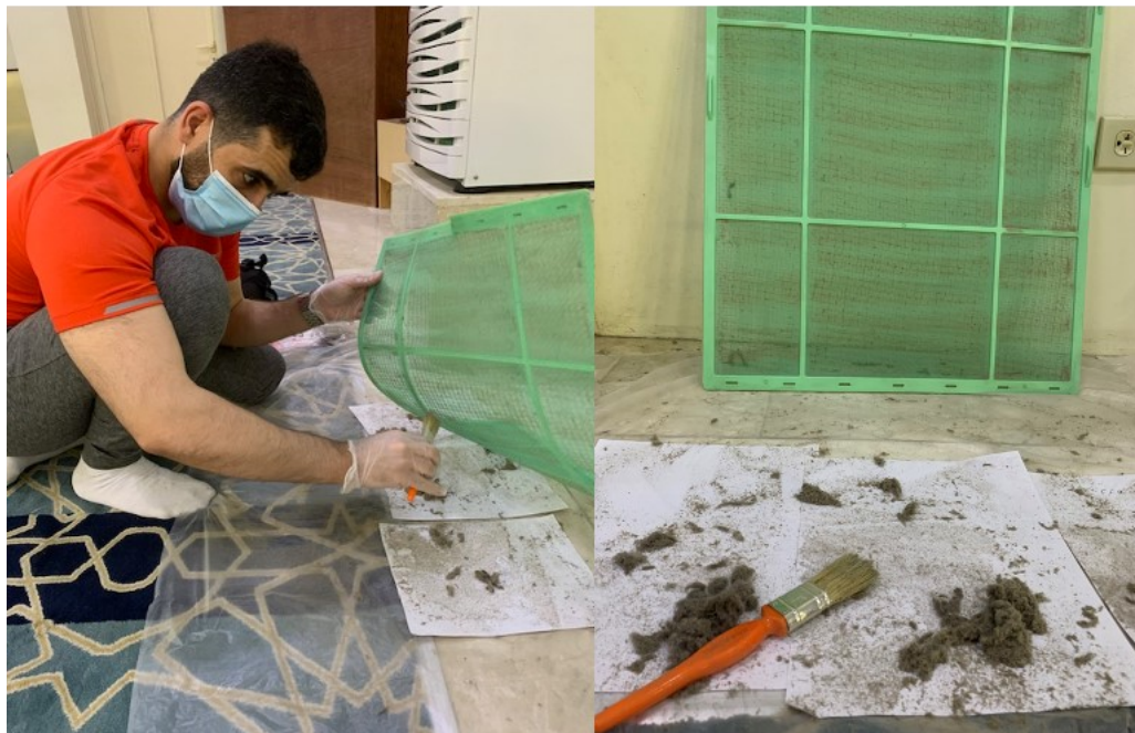
Figure 4 Main step of collecting dust from AC filters.
