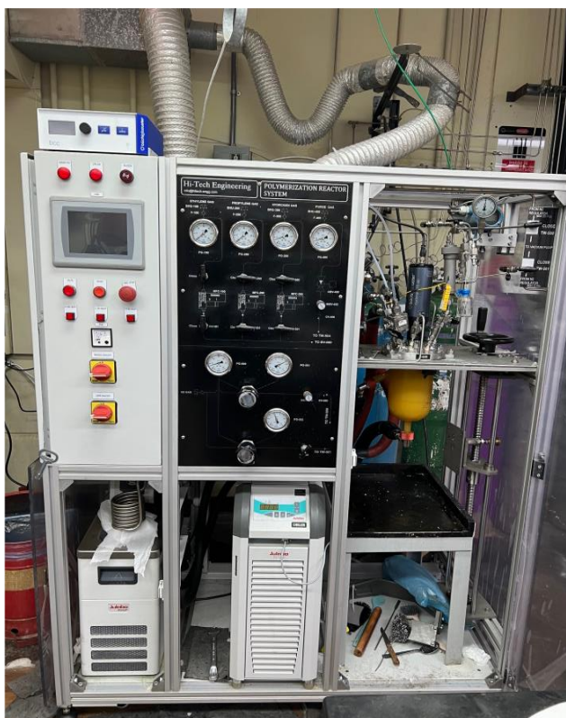
Figure 4.9: Computer-operated HighTech polymerization reactor system.
