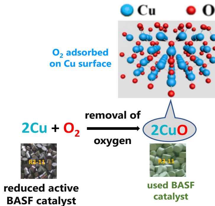
Figure 4.2: O_2 removal mechanism by BASF adsorbent catalyst.
