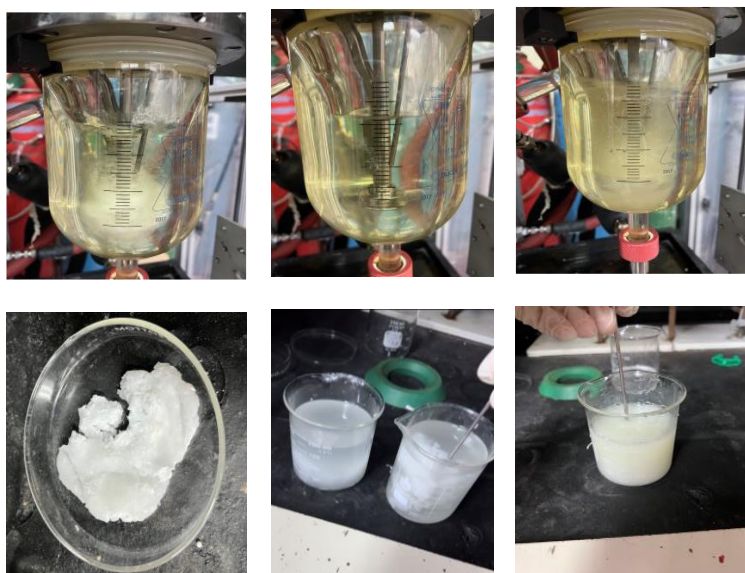
Figure 4.10: Separation and purification of as-synthesized elastomers.
