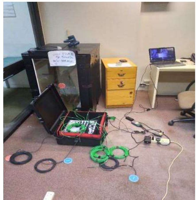
Model 03 setup and heat flux wiring
