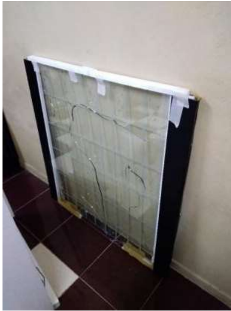
Testing window in extremely high temperature of at 80 °C
