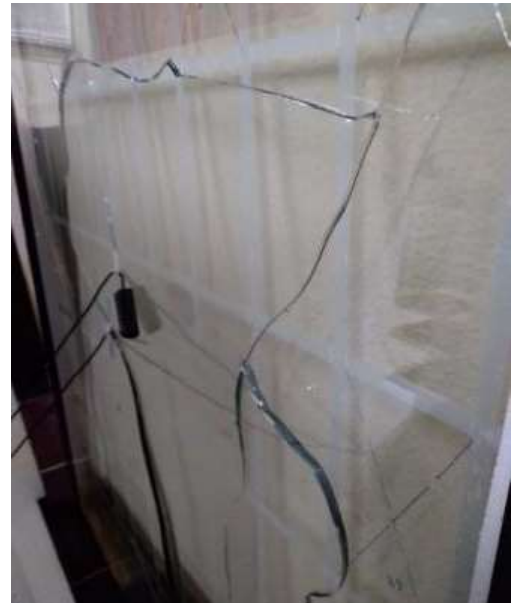
Testing window in extremely high temperature of at 80 °C, closer shot
