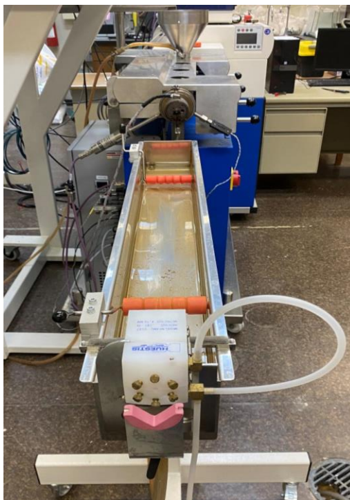
Figure 11 Water bath to cool the extruded polymer strand as it emerged from the die
