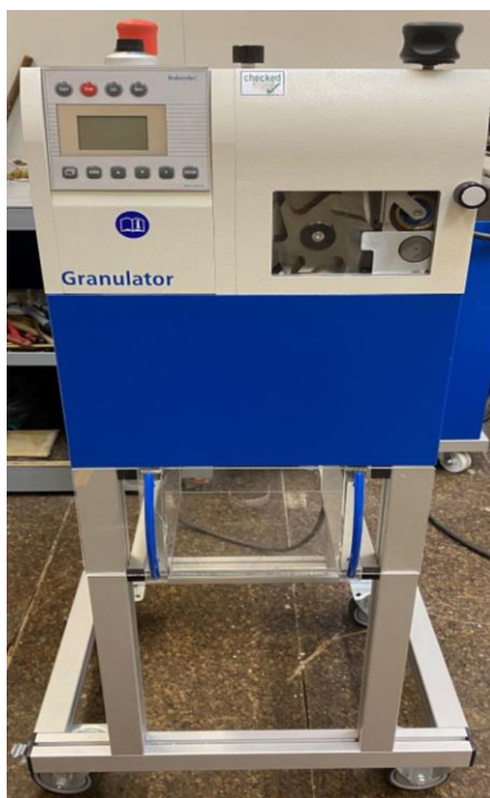
Figure 12 Granulator to pelletize the cooled polymer strand
