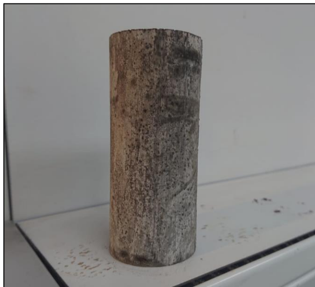
Figure 8.3 VT-based geopolymer cured sample after 24 h at 200°F.
