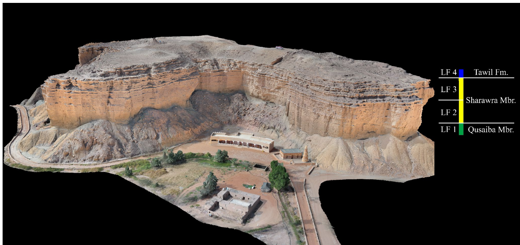
Figure 16 Digital outcrop model (DOM) of outcrop 1 (OC1; Figure 2) illustrating stratigraphic architecture. The lowermost unit is the Qusaiba Member (LF 1), overlain by the Sharawra Member (LF2 and LF 3), and capped by the Tawil Formation (LF 4). Please note that the Tawil Formation is mostly eroded and is limitedly exposed. This high-resolution DOM provides a detailed representation of the large-scale sedimentary structures, bed geometries and lithological variations within the outcrop facilitating geological interpretations, and static models.
