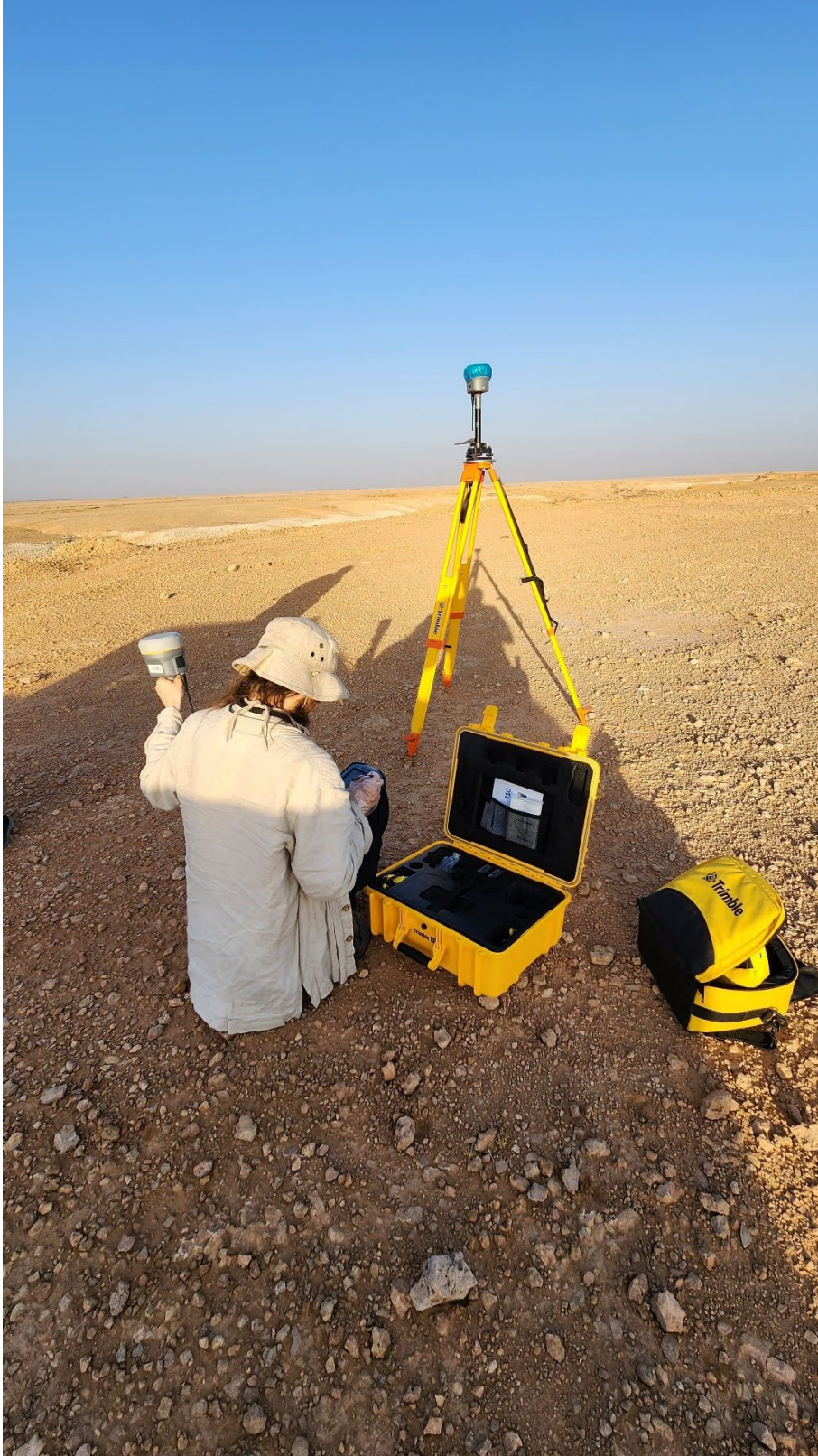
Figure 6 Showing the Trimble R10 device
