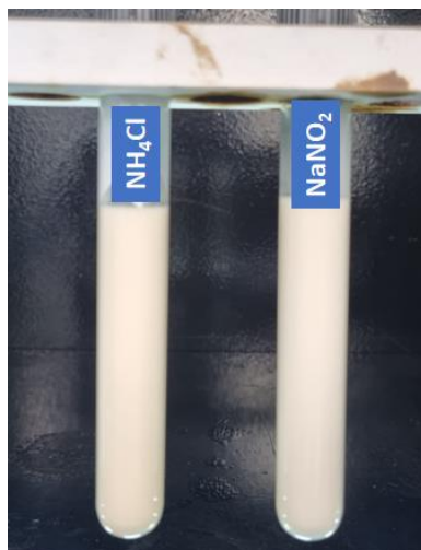
Figure 4.16-Photos of individual emulsified 50% TCFs in diesel with 1% Emulsifier-A after viscosity measurement cycles of 25 to 90°C
