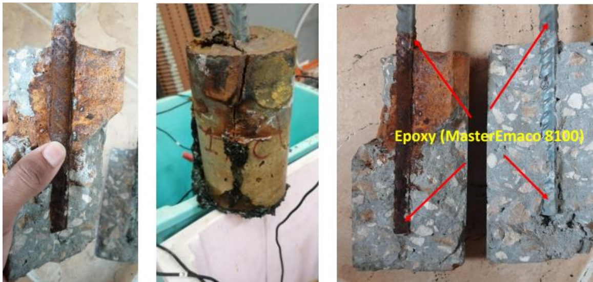
Figure 17 corroded and uncorroded tests samples
