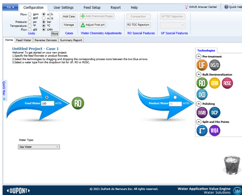
Figure 4.3: WAVE RO design software from Dow [52]
