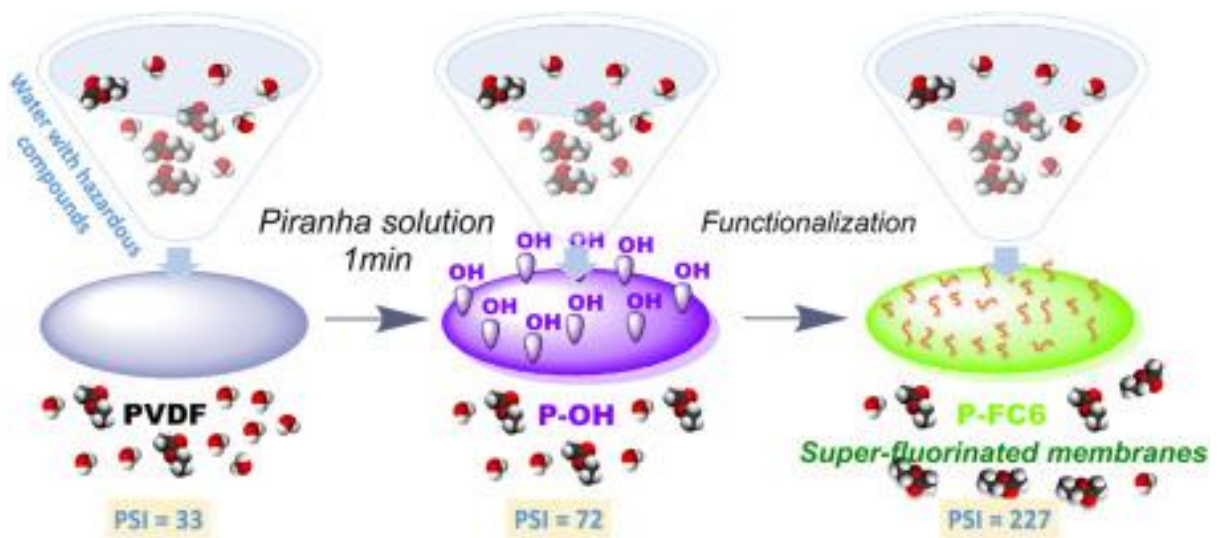
Figure 13 :VOCs removal membrane
