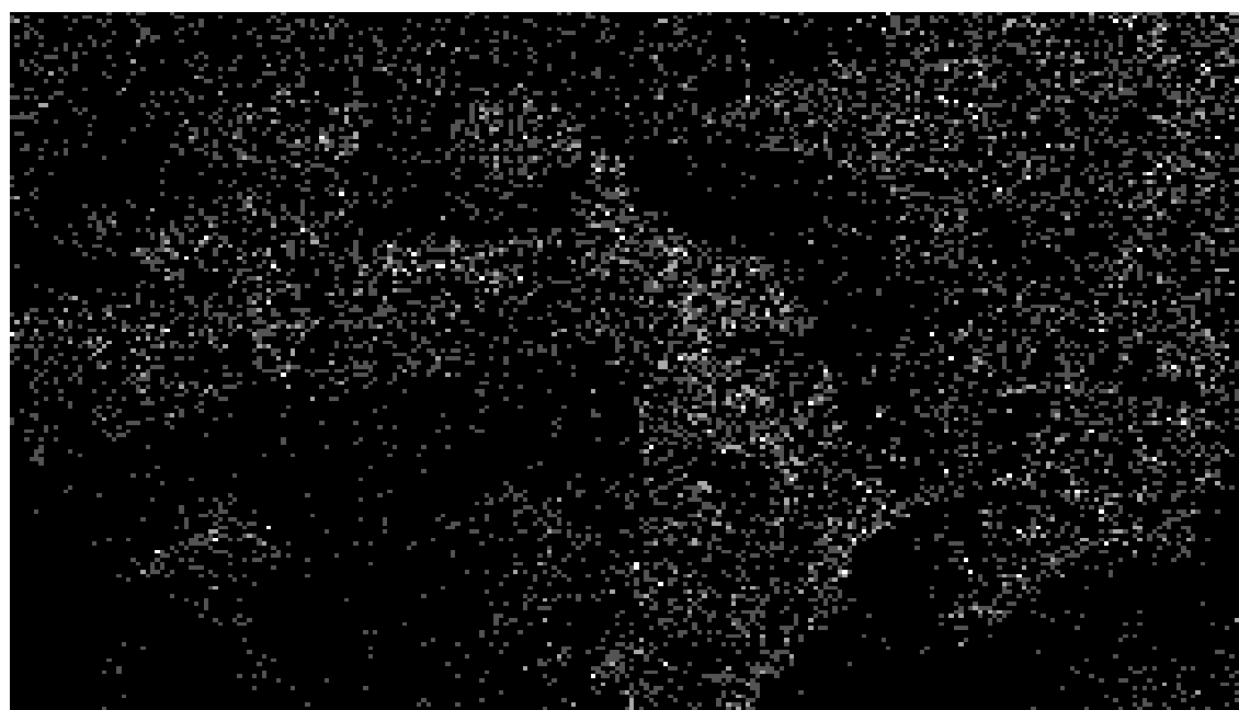
Figure 16: SEM mapping image of gold element (used to coat the sample during SEM imaging) in the polyacrylate-modified CNT.
