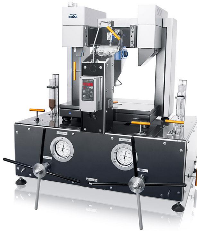
Figure 5- Drop shape analyzer used for contact angle measurements
