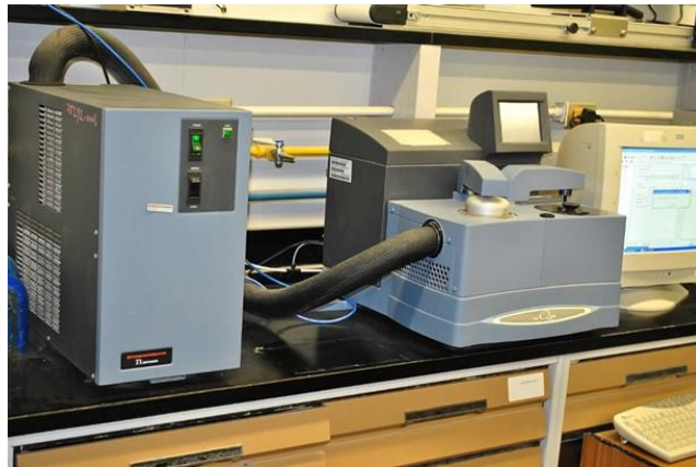
Figure 3.5: (DSC) Q2000 V24.9 TA instruments® machine
