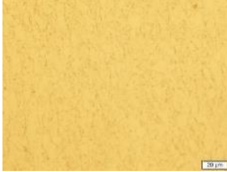
Figure 49: Microstructure of the as received TMCP material and heat treated at 650 °C.
