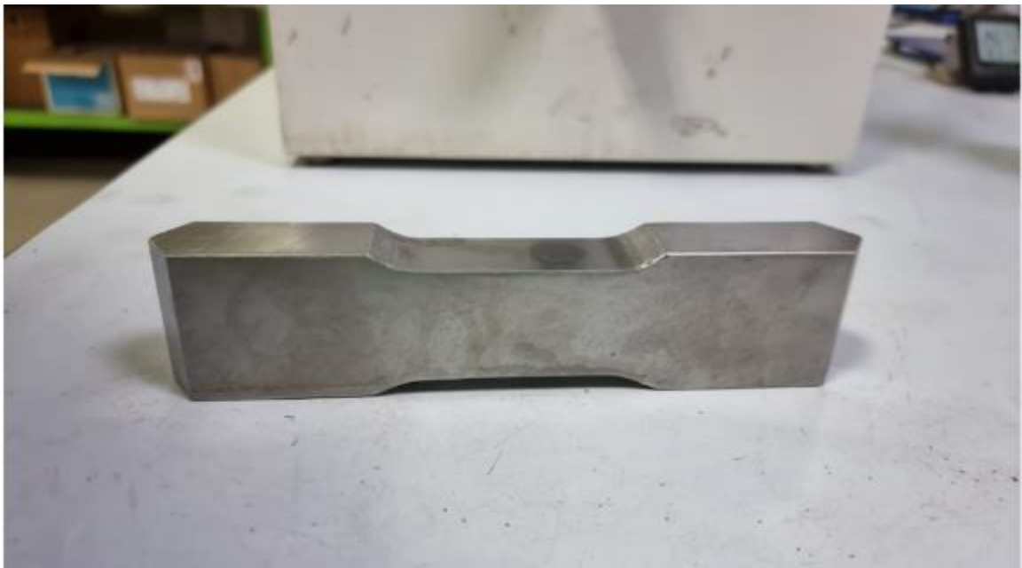
Figure 39: Tensile Test Specimens prior to immersing in the NACE solution A.
