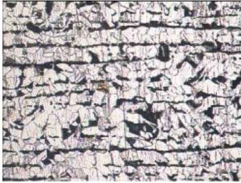
Figure 50: Reported microstructure of carbon steel ASME Process Piping SA106 Grade B in the as received and heat treated conditions [67].
