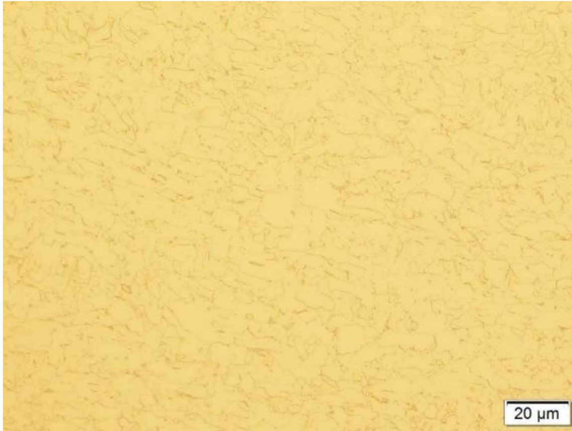
Figure 54: Microstructure of as received sample which shows ferrite pearlite microstructure (5% Nital etched. 500X magnification).
