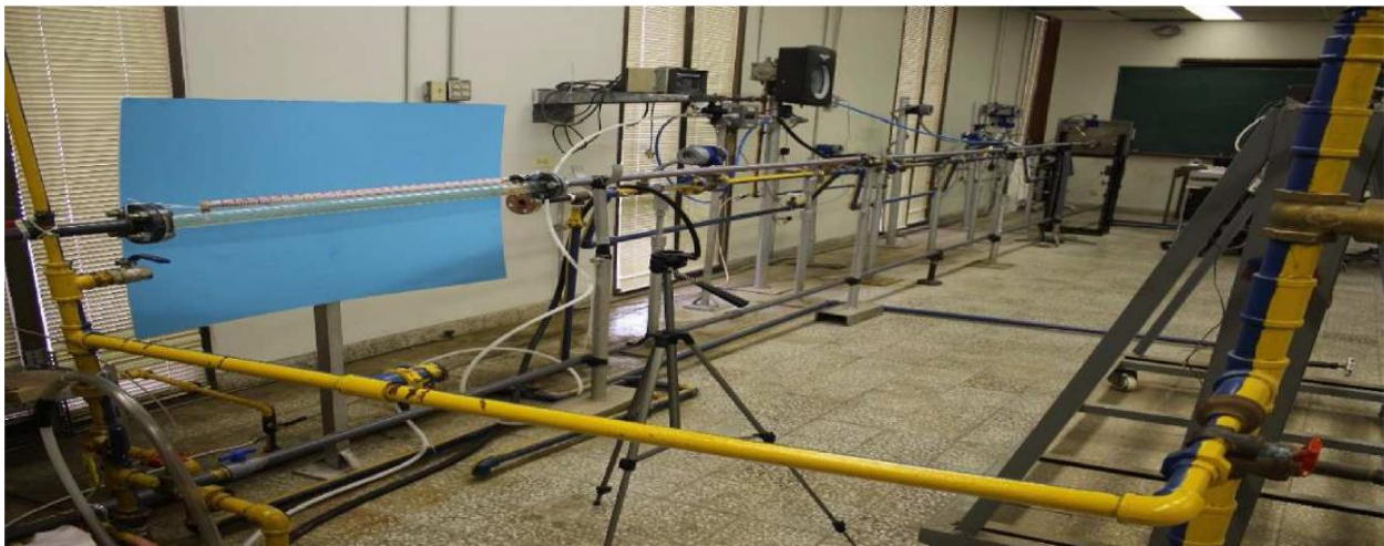
Figure 1 Horizontal Flow Loop[1]
