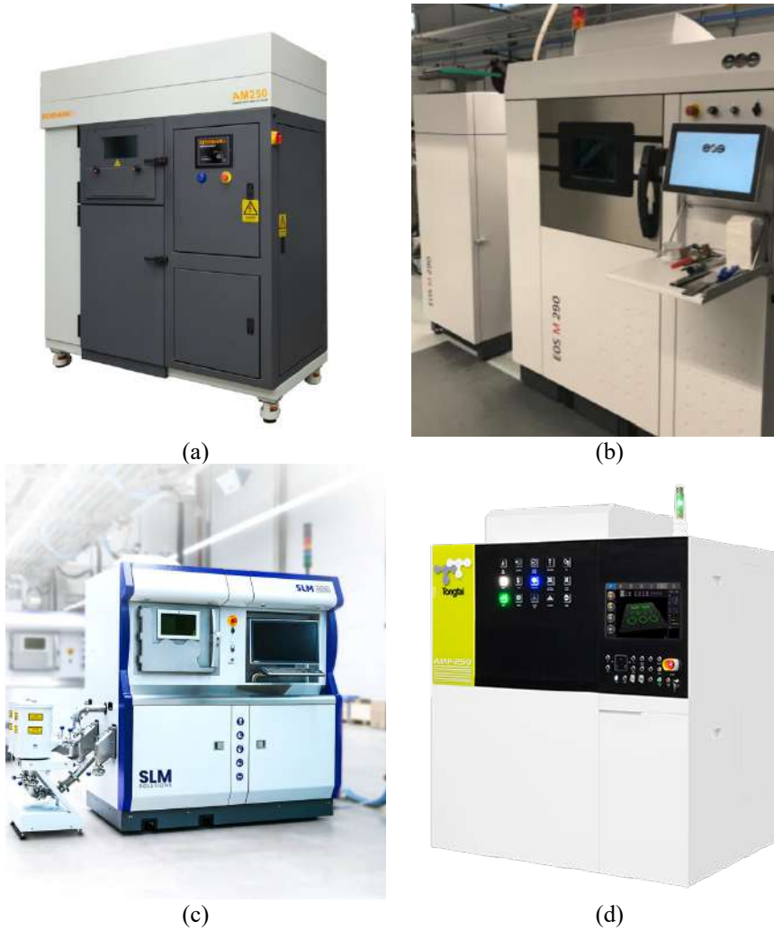
Figure 2.3: Laser powder-bed fusion machines used for experimental studies (a) Renishaw AM250 [50] (b) EOS M290 [49] (c) SLM Solutions 280HL [51] (d) TongTai AMP 250 [52]
