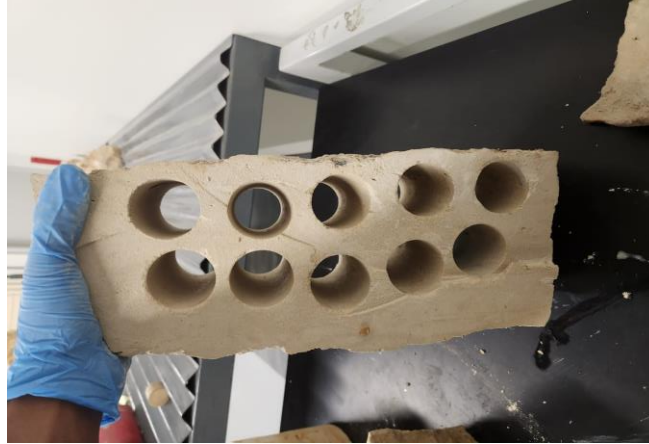
Figure 3-13 Cores extraction from outcrop rock sample after slabbing.
