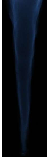
Figure 28: Blowout condition at 0% HF.
