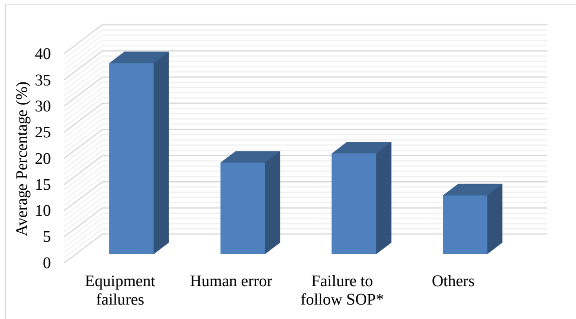
Figure 10: The potential causes of pipeline failure incidents in hydrogen transportation.
