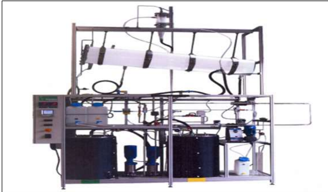
Figure 1 A 3D image of the drag duction flow loop system (Khalid et al., 2020)
