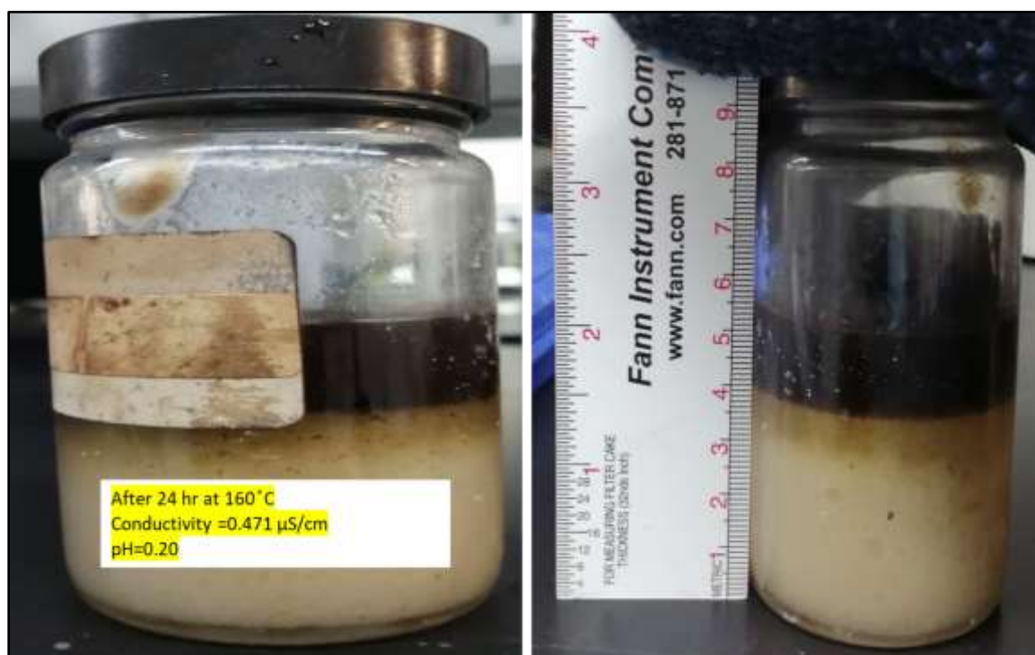
Figure 43 Stability of Pickering EAS prepared with 500 ppm of Claytone-IMG 400 after 24 hr at 160 °C
