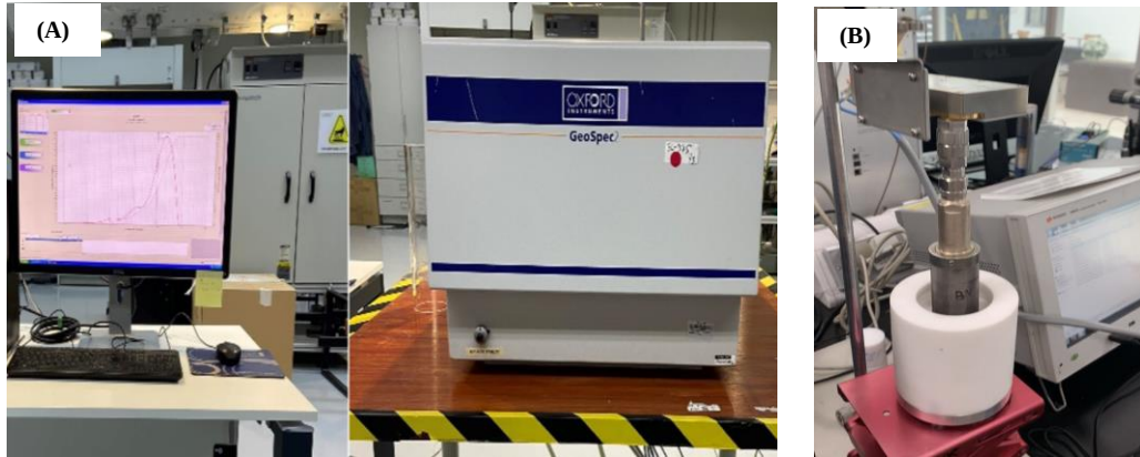
Figure 30 The NMR rock analyzer (A) and the multifrequency dielectric instrument (B) used in the study.
