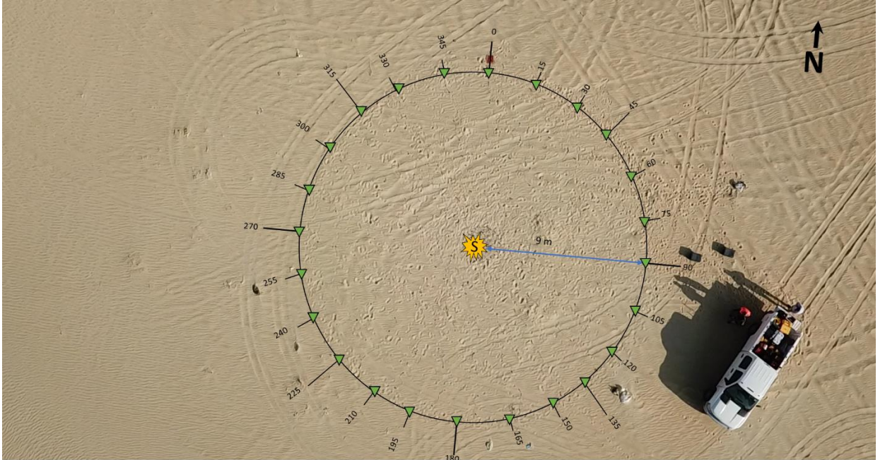
Figure 25: Areal view of the study area with an illustration of the seismic array geometry, with a point source (demarcated by orange star) in the center of the 9-m radius circle and the 24 geophones (demarcated by green triangles) and their azimuth relative from north.
