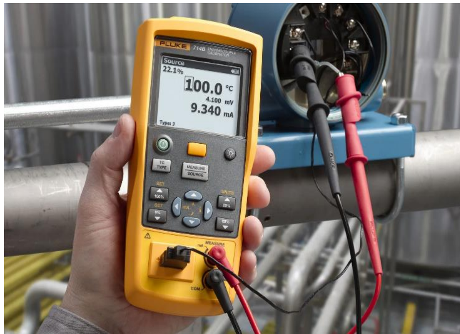
Figure 1.3: Physical technique of temperature measurement using thermocouple [14].
