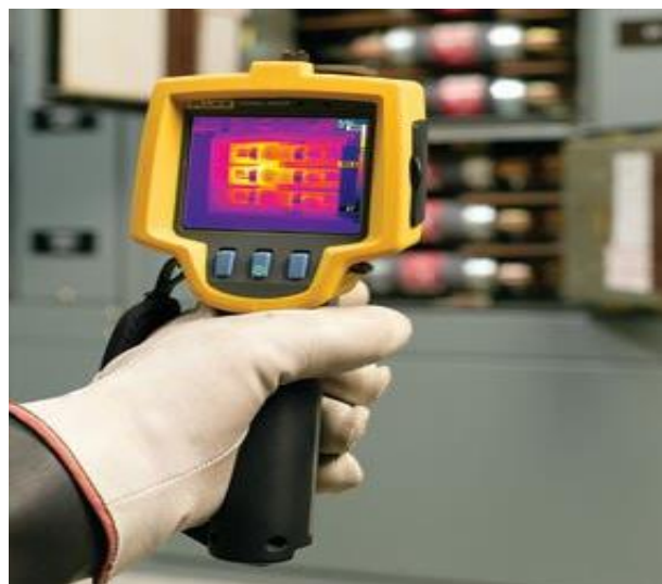
Figure 2.13: Temperature sensing using IR camera [61].
