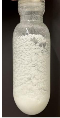
Figure 3-5 White precipitation for Baseline, cellulose and AM-AMPS at 120°C
