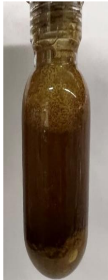
Figure 3-6 Dark precipitation of degraded xanthan gum at 120°C
