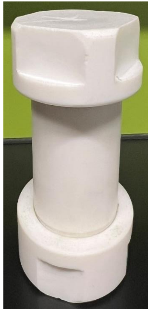
Figure 3-9 Teflon container for 120°C
