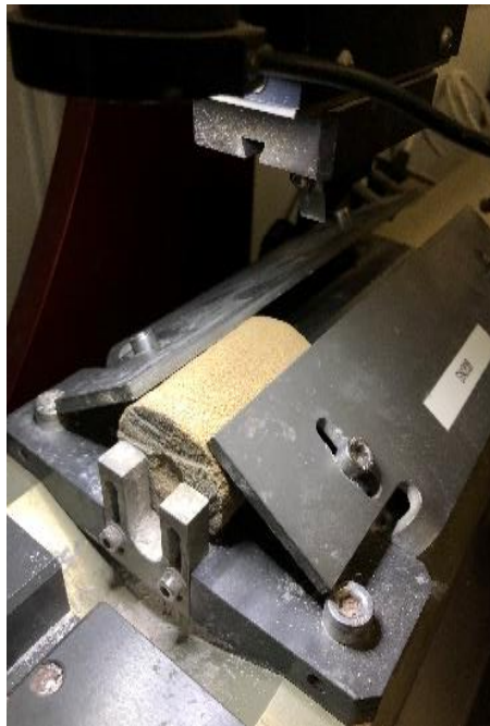
Figure 3-13 Scratch test machine (Epslog)
