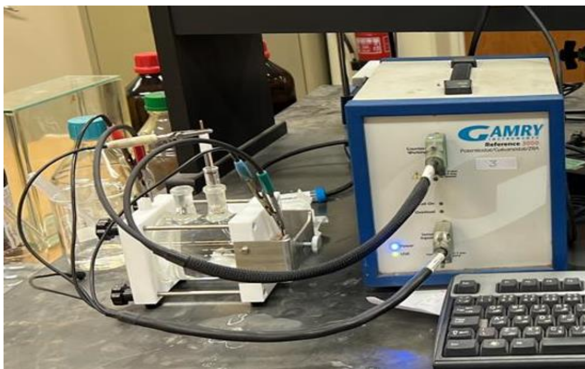
Figure 16: electrochemical test set up for the room temperatures.
