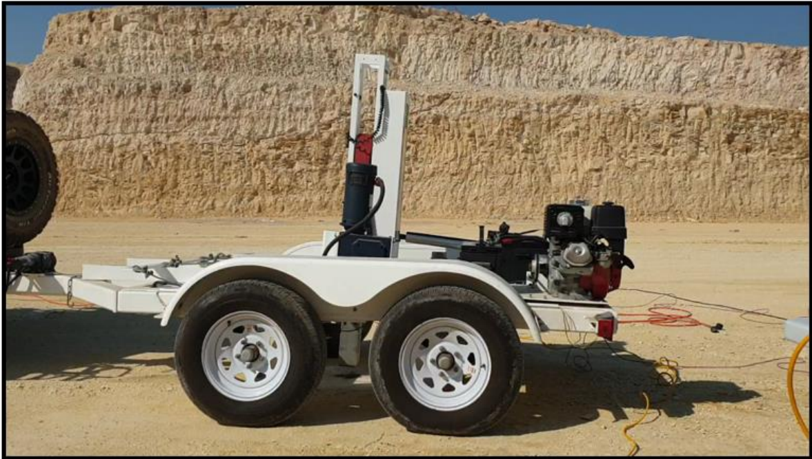
Figure 15: Shows the source which has been used in both 2D and 3D seismic acquisition which is acceleration weight-drop. The source is capable of generate P- wave as well as S-wave with only tilting the hammer in different angel, or keeping it perfectly vertical to generate P-wave.
