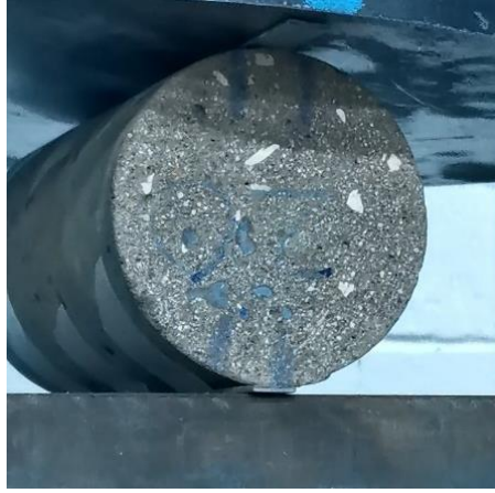
Figure 5-2 Split-tensile strength test setup
