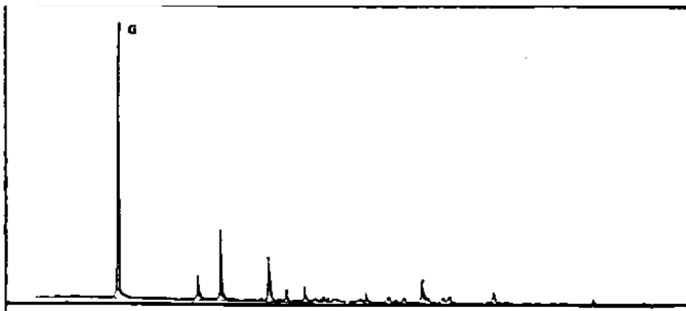
Figure 3-9 XRD analysis of gypsum (G: Gypsum)[151]
