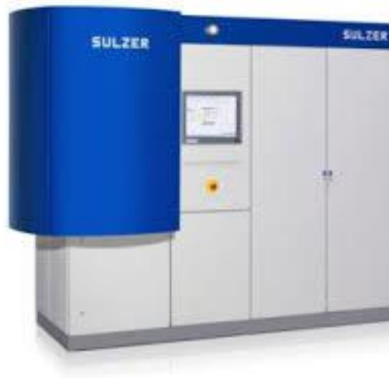
Figure 3.2: The image of the cathodic arc evaporation equipment
