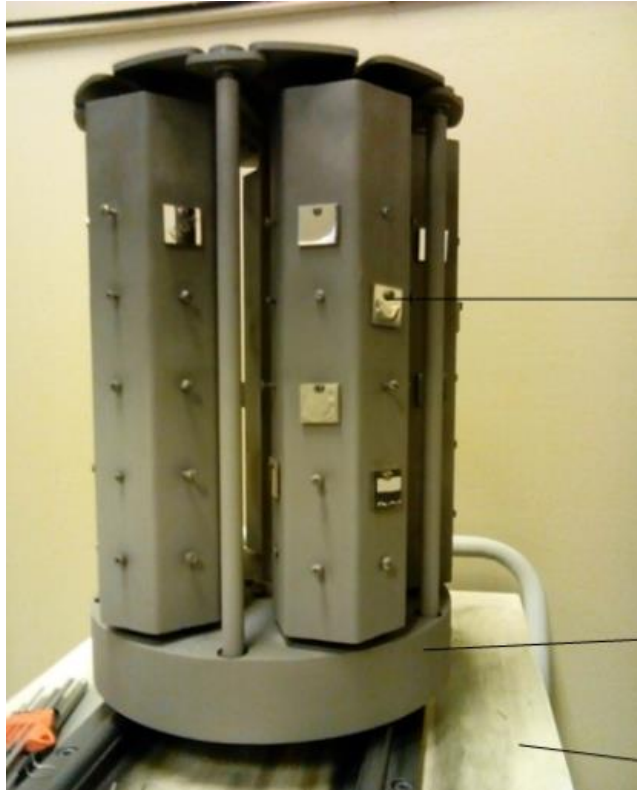
Figure 3.4: Samples loaded in the planetary lift car
