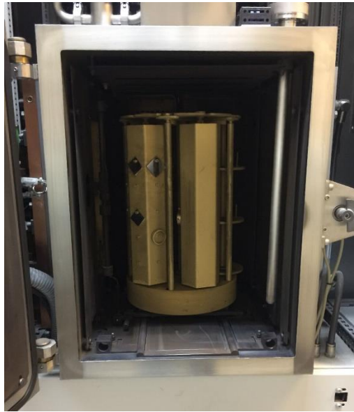
Figure 3.3: The loaded samples inside the chamber of the cathodic arc evaporation
