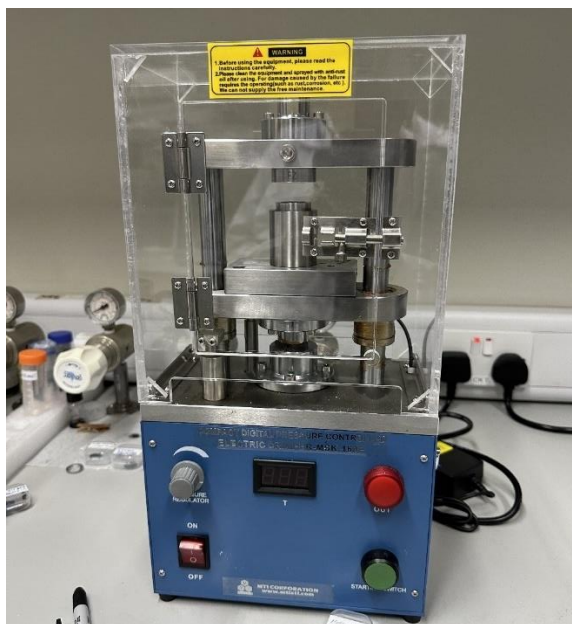
Figure 21: Pressure controlled crimper used for coin cell fabrication.
