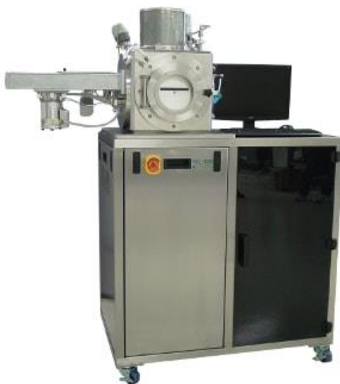
Figure 23: Sputtering setup for the fabrication of VO cathode material.
