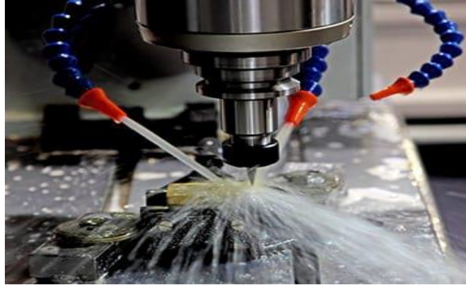
Figure 1.10 Flooding cutting fluid technique in the end milling process.
