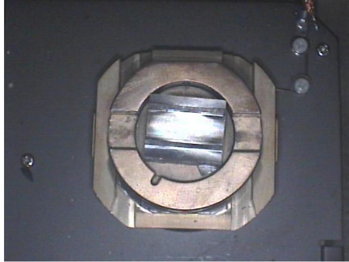
Figure 4.7 Machined sample under CNT nano-oil is inside SEM chamber.
