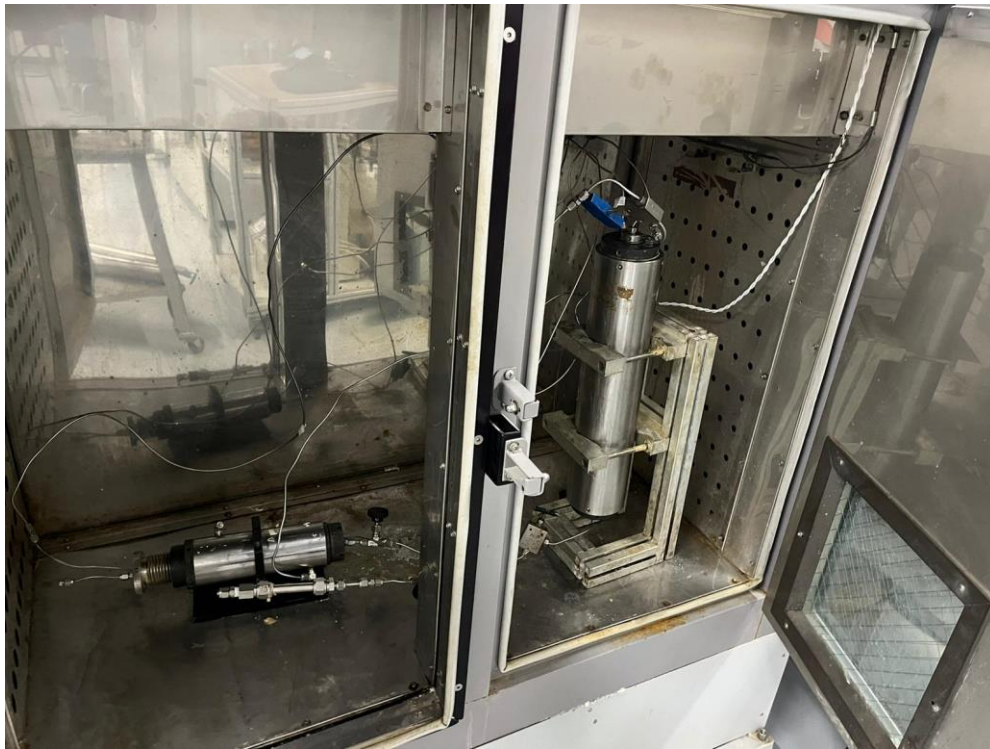
Figure 27: The core holder attached to the live brine accumulator inside the oven.
