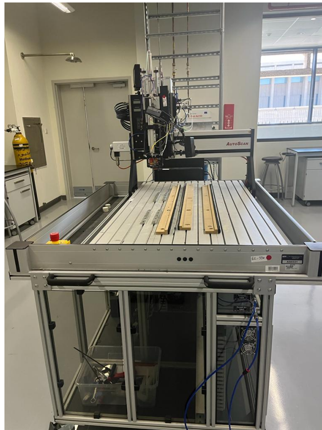
Figure 22: Hardness measurements using a non-destructive AutoScan scanner
