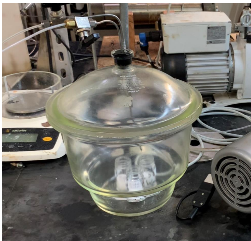
Figure 28: Illustration of saturation desiccator setup
