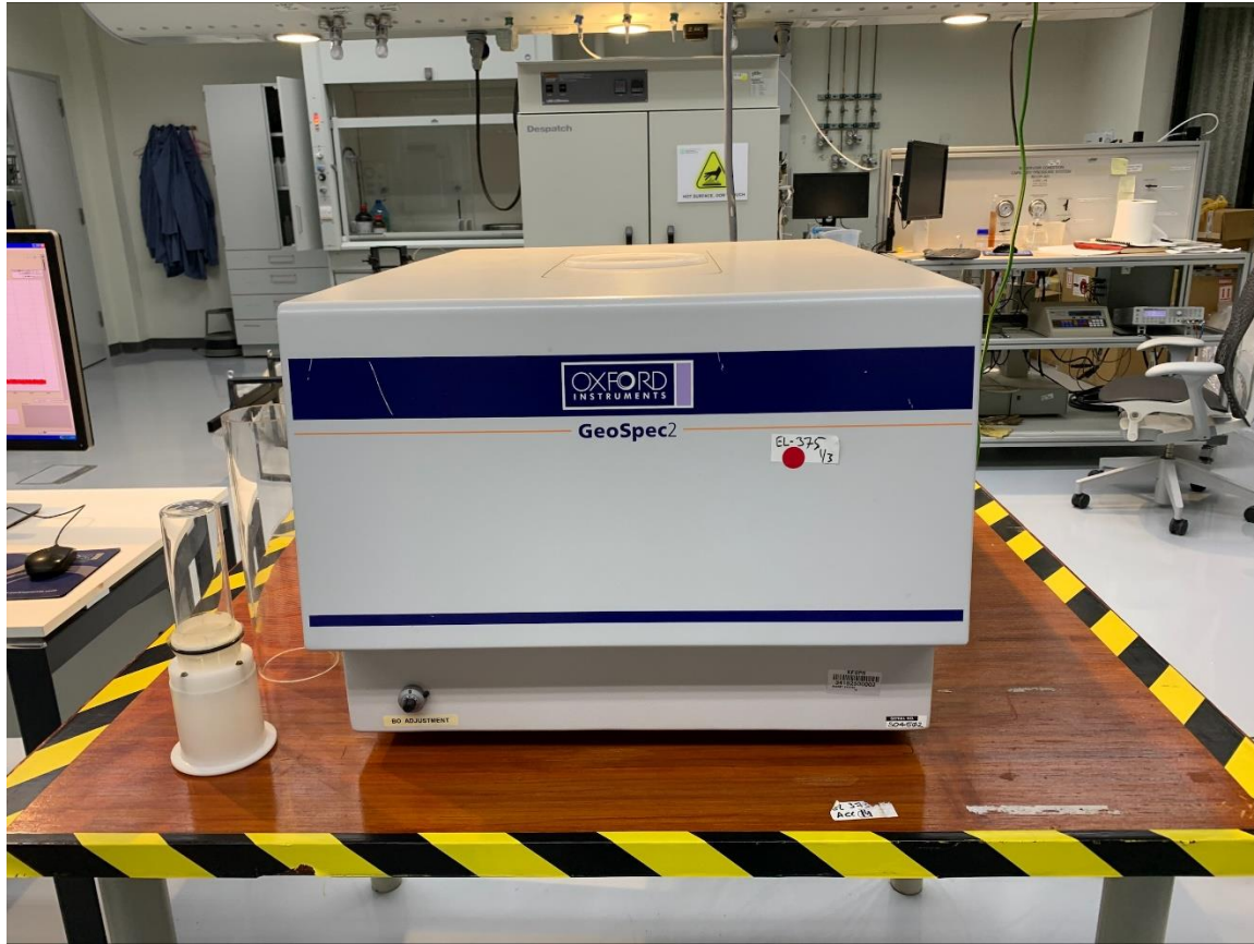
Figure 35: NMR Oxford 2 MHz Geo-Spec 2, which was used in the laboratory work.
