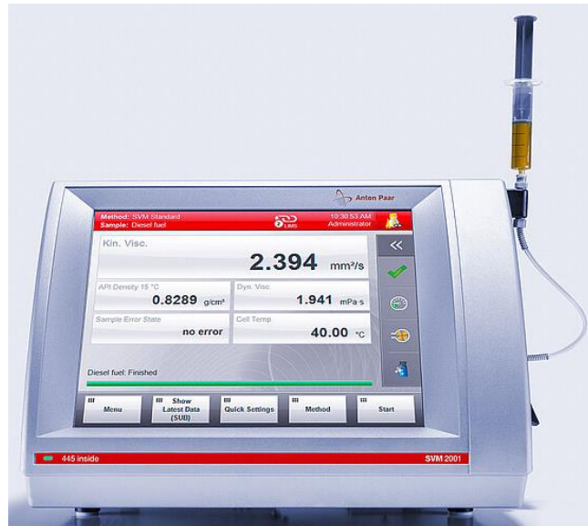
Figure 25: Anton Paar SVM 3001 Stabinger viscometer used to measure fluid properties
